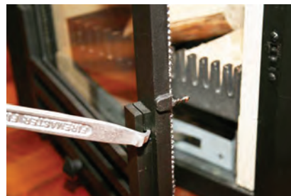
(Fig 15a) Opening and closing the door
