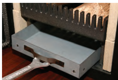
(Fig 15b) Removing ash pan
