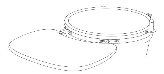
STEP 16 - Insert the 2x table hinge into each of the table brackets (23 & 24).
