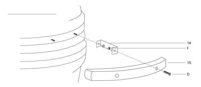
**STEP 10 -** To attach the handle (15) to the lid of the Kamado Grill (12) start by attaching 2x handle brackets (14) using the 2x pre-attached bolts and dome headed nuts. Attach the handle (14) to the brackets (16) using 2x bolts (D) and nuts (F)
