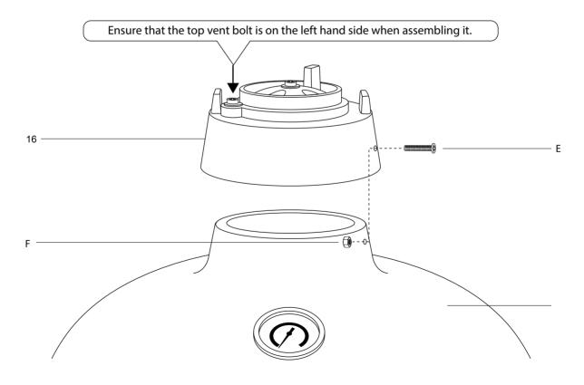
**STEP 11 -** To attach the top vent (16) to the Kamado Grill (12) place it on top and align both the bolt holes. Secure using 2x bolts (E) and nuts (F). Ensu re that the top vent bolt is on the left hand side when assembling it.
