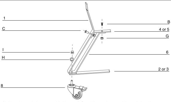
STEP 2 - (Joining the two halves assembled in step I) Stand the section 1 upright, and place the upper cross braces (4&5) close to section 1. Inserting truss head screw C through the hole of section1 and section 4&5 and install G Keps nut and tighten securely.
