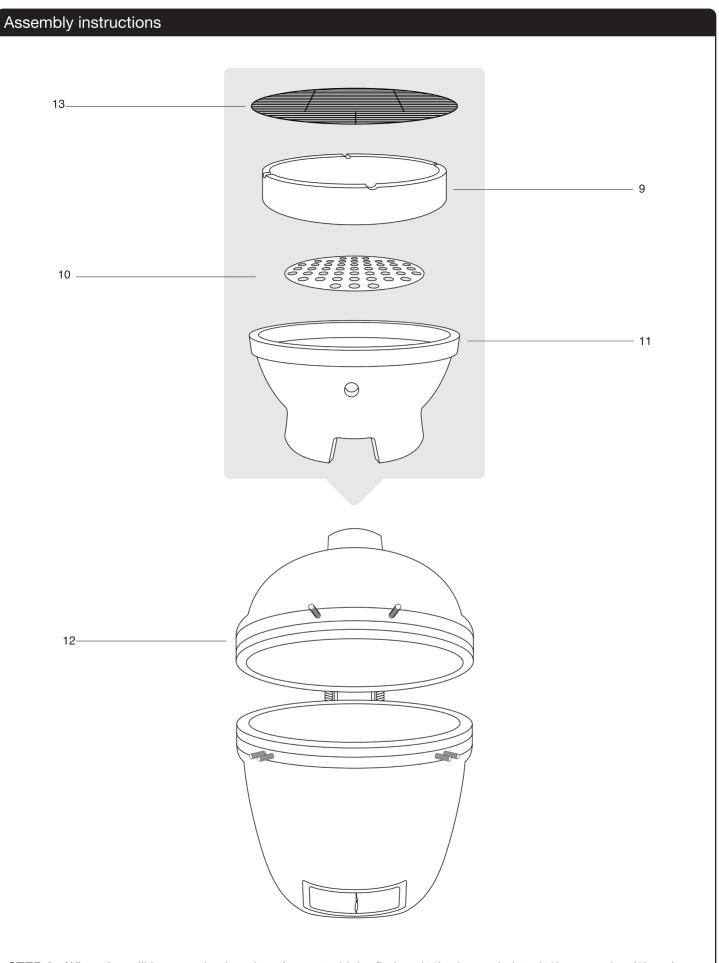
STEP 8 - When the grill is securely placed on the cart add the firebox (11), charcoal plate (10), upper ring (9) and cooking grill (12) inside of the Kamado Grill as displayed in the assembly diagram.
