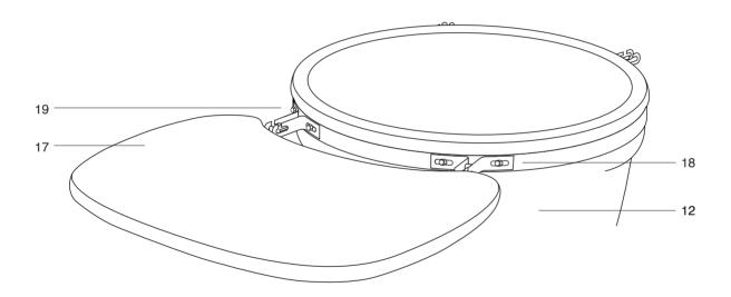
STEP 14 - Insert the 2x table hinge (17) into each of the table brackets (18 & 19).
