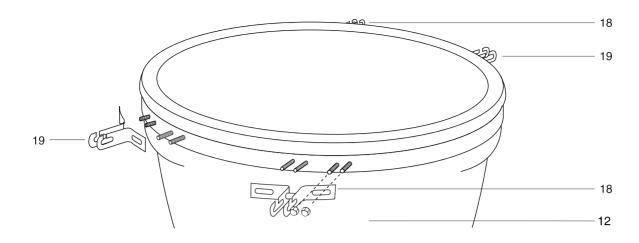
**STEP 12 -** Attach the 2x table brackets (18) to the Kamado Grill (12) using the 4x pre-attached bolts and dome headed nuts per bracket. Please note the position shown in the above diagram.
